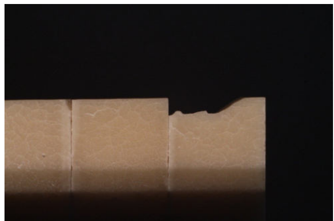
Fig. 32. Material failure on Ketac Fil test specimen under 1.2 N press force.
