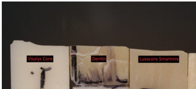
Fig. 34. Depth comparison between Visalys Core, dentin and Luxacore Smartmix under 1.2 N press force.
