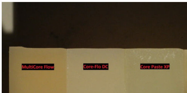
Fig. 35. Depth comparison between MultiCore Flow, Core-Flo DC and Core Paste XP under 0.5 N of press force.
