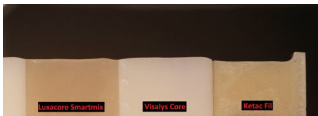
Fig. 14. Removal depths of Luxacore Smartmix, Visalys Core and Ketac Fil under 0.5 N of press force.
