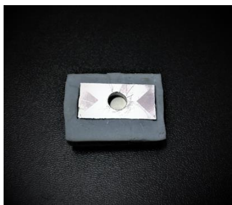
Figure (12) Adhesive bonding through the aluminum jig
