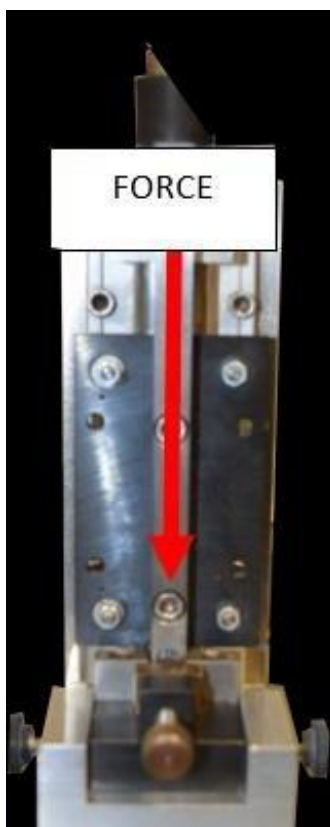
Figure (26) Direction of force on specimen in universal testing machine
