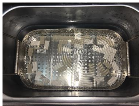
Figure (7) Ultrasonic cleaning in 70 % ethanol
